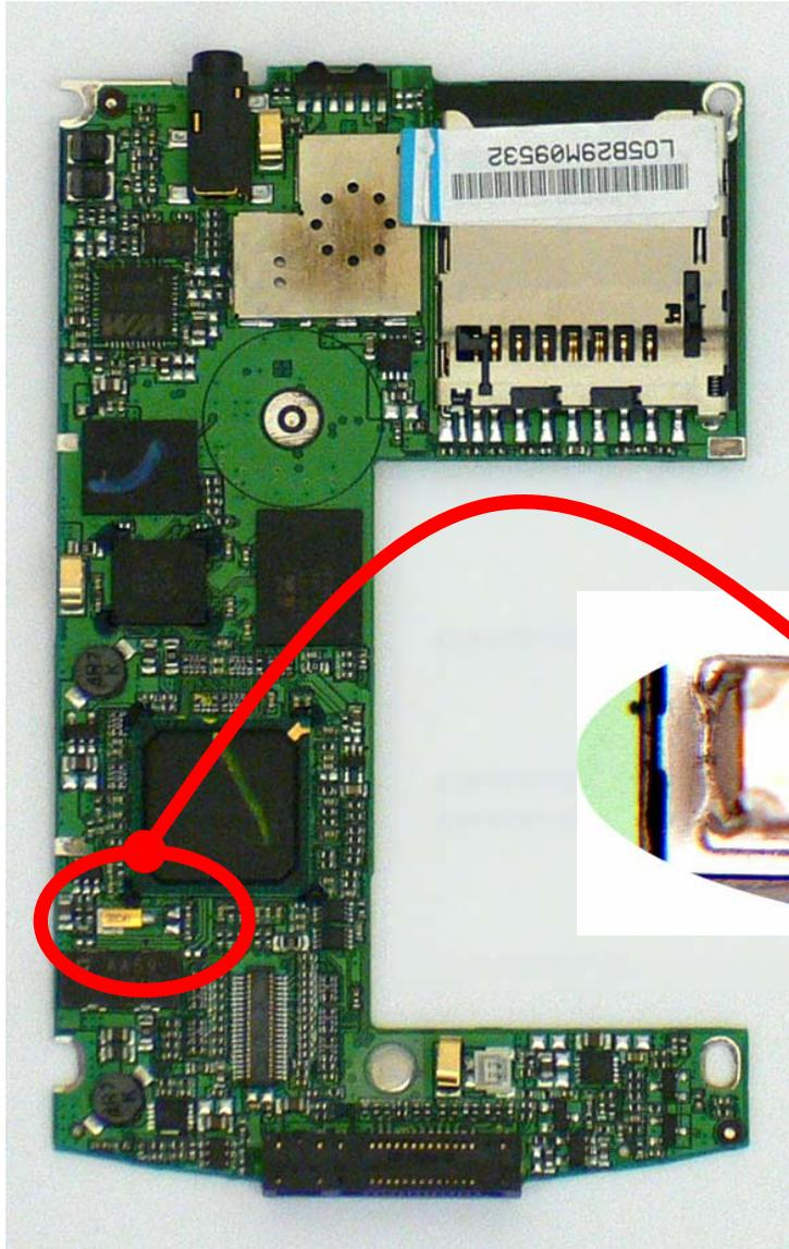
Analysis of these solder pads for ceramic crystals on PCBA may reflect the high temperature / **high Pb solder**. This is currently allowed per RoHS Exemption #7.
