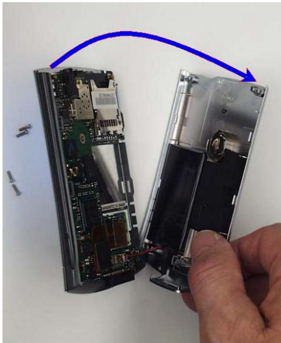
TE2.07 REMOVE TOP, BUTTON AND BATTERY CONNECTOR
