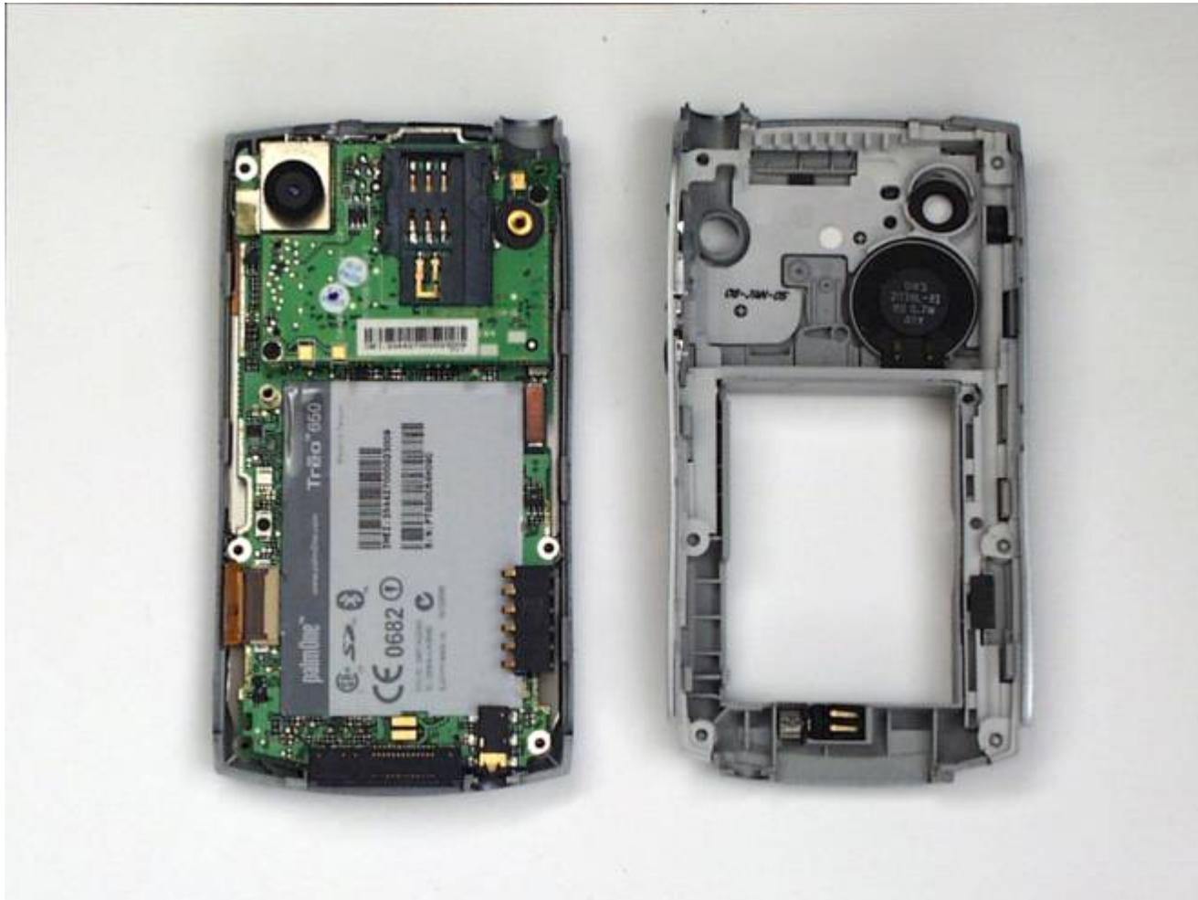
T650.10 REMOVE BUTTON AND VIBRATOR, PRY SPEAKER,
