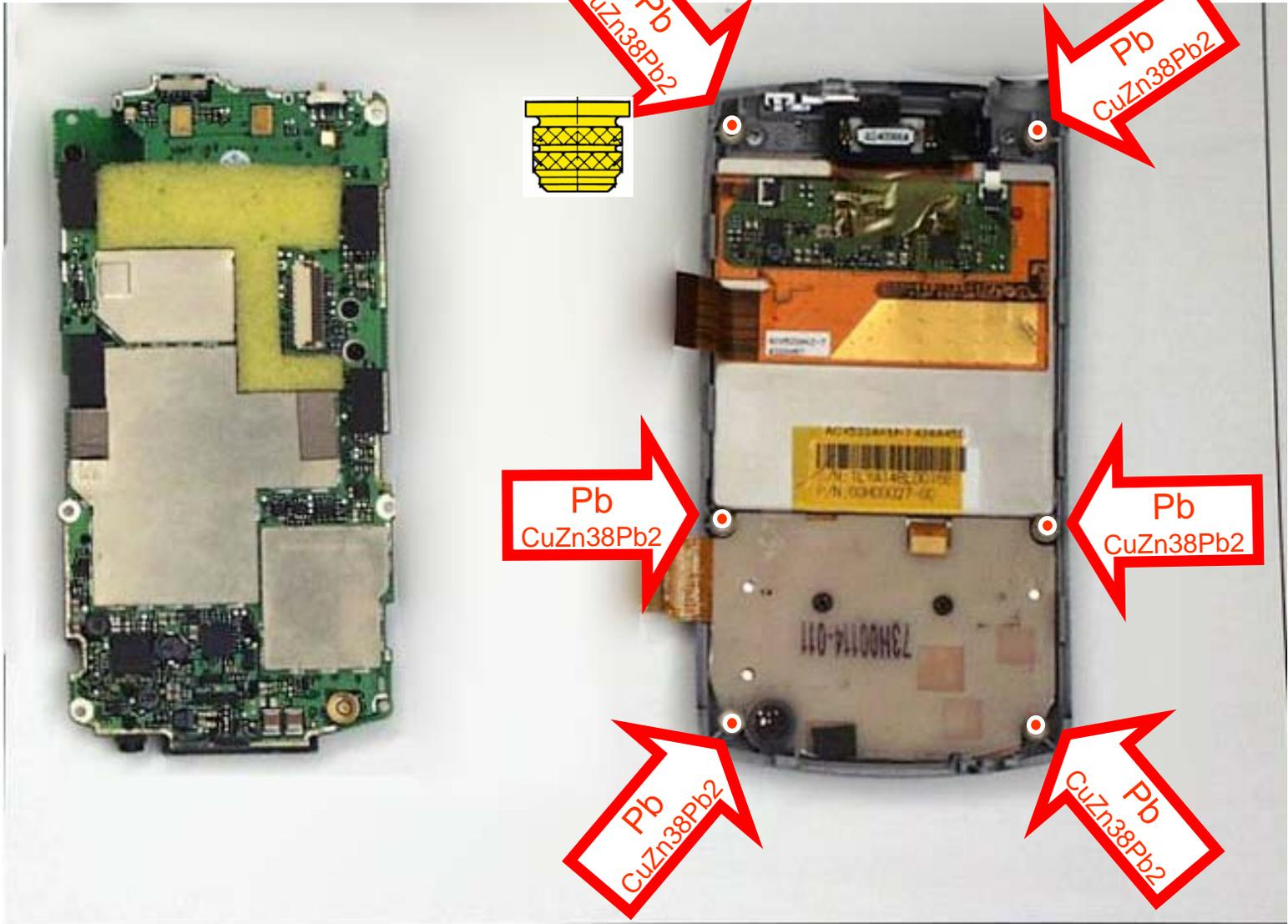
T650.13 REMOVE LCM, VIBRATOR AND RECEIVER, KEYPAD SCREWS
