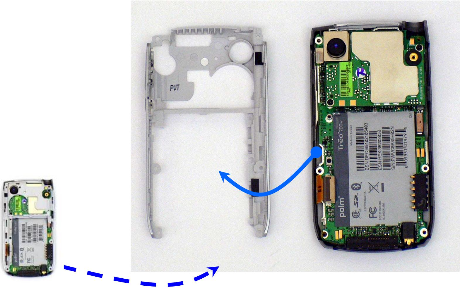
T700.12 REMOVE PCBA AND LCM; NOTE BRASS INSERTS (6)
